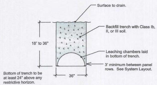
There shall be 12" of fall between the invert of the septic tank outlet and the trench bottom, min.
